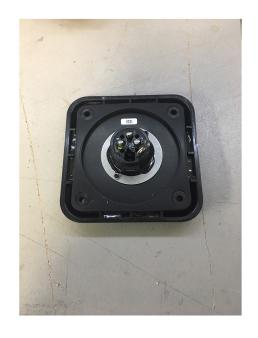
Lift shock mount up and flip over from the bottom upwards and over so the single solder point is at the top and pair of solder points are oriented on the bottom, as shown.
