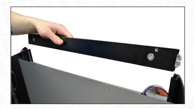
Using T30 torque wrench, loosen torque screws holding the cross beam in place.
